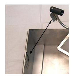
The bracket fits into a slot in the pan.
